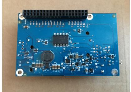
Integral PSU: 5V @ 2A, 2.4MHz switching, 96% efficiency
